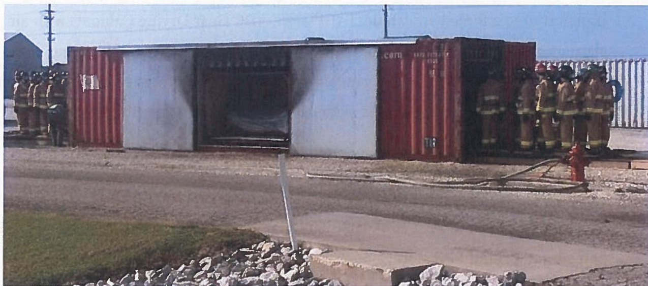
Fireground smoke exposure (FES) prop preparing for mannequin-based exposure testing [17]
