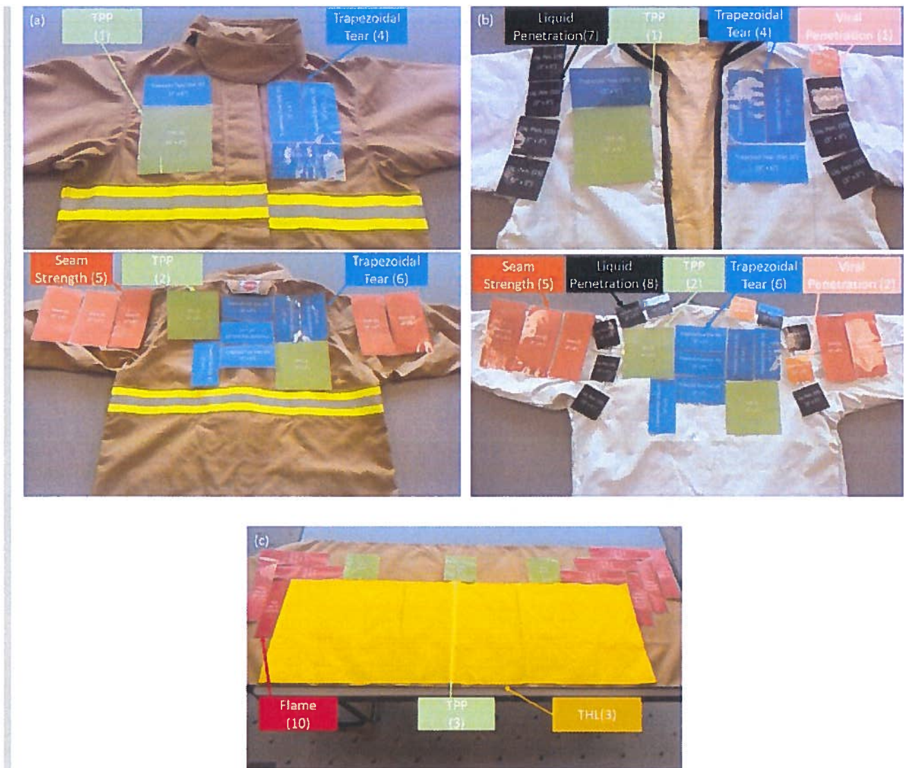
(a) Shell specimen locations at the front (top) and back (bottom). TPP (3), Tear (Warp, 5; Fill, 5), Seams (5); (b) moisture barrier and thermal liner specimen locations at the front (top) and back (bottom). TPP(3), Tear (Warp, 5; Fill, 5), Seams(5). For moisture barrier only Liquid Penetration (15), Viral Penetration (3); (c) blanket specimen locations at the front (top) and back (bottom). All three layers—TPP(3), THL (3). For shell only Flame (Warp, 5; Fill, 5)
